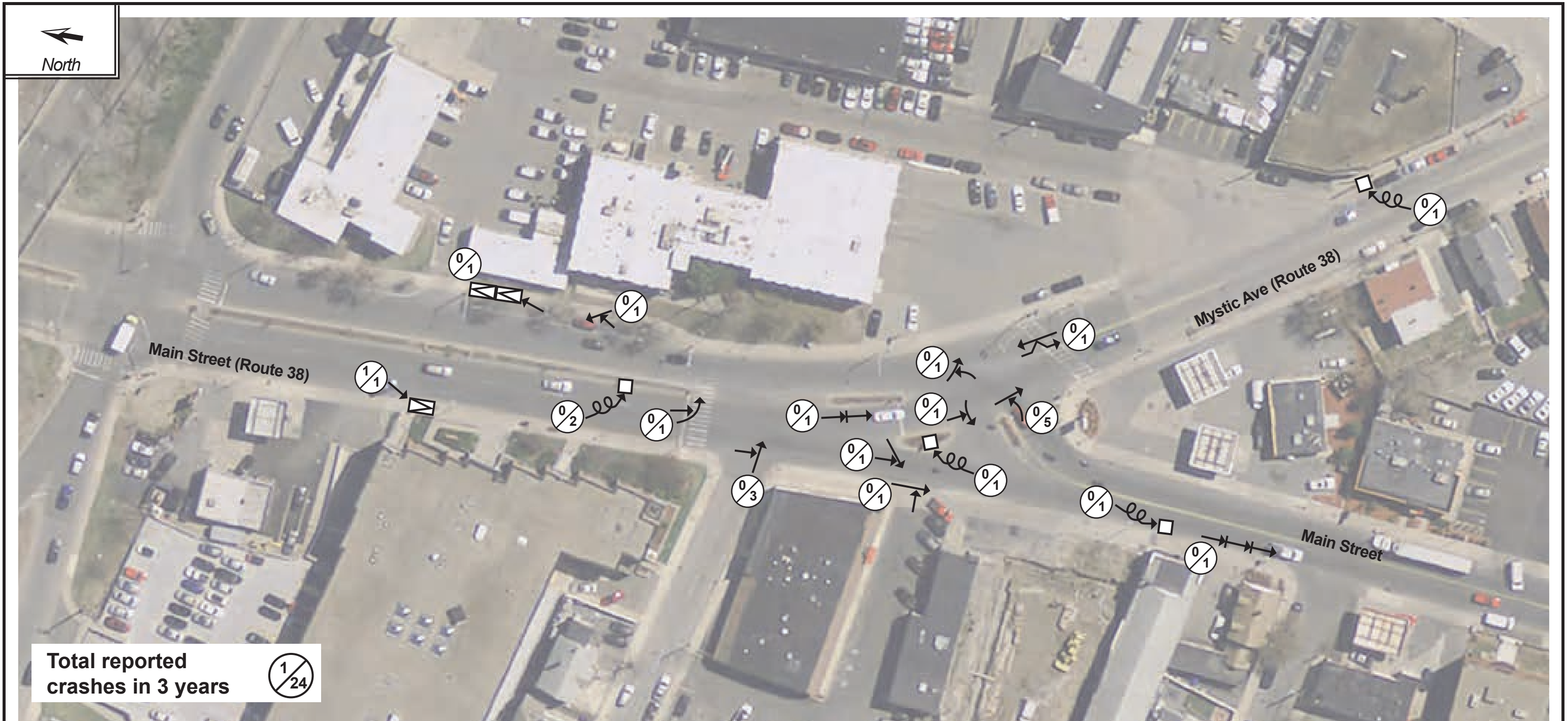
Figure 8 Collision Diagram: Main Street at Mystic Avenue Medford Police Reports: January 2015–December 2017
